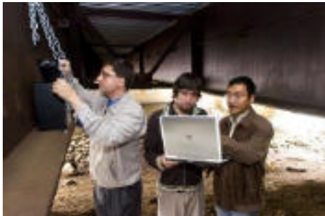
Clarkson University Assistant Professor Edward S. Sazonov and graduate students Darrell Curry and Haodong Li check data from a wireless bridge sensor on the Route 11 bridge in Potsdam, N.Y. Clarkson researchers have developed technology that uses the vibrations caused by passing traffic to power wireless bridge monitoring sensors. (Credit: Clarkson University photo by Christopher Lenney)
